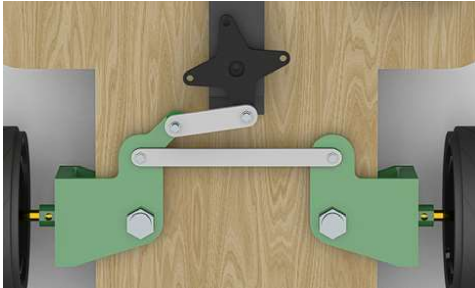
Figure (1): Ackerman Steering System, Joint linkage
