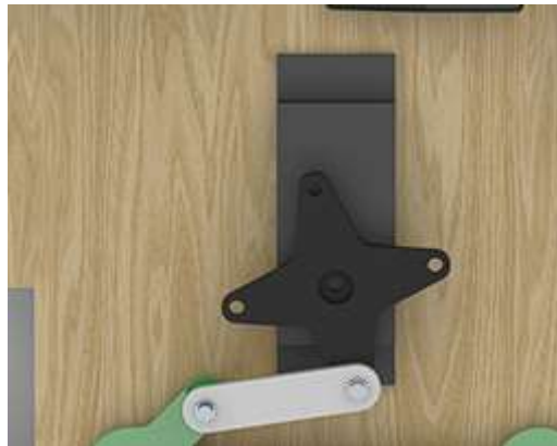
Figure (2): Ackerman Steering System, servo head mount
